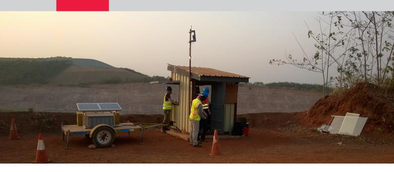
Mining engineers and geologist use the results of this monitoring solution to understand the behaviour, condition and movement of a mine. If something moves, professionals using this software will know immediately. Detecting such movements around-the-clock also provides a continuous, long-term picture to form a better understanding of the pit's walls, which are continuously being chipped away at.
